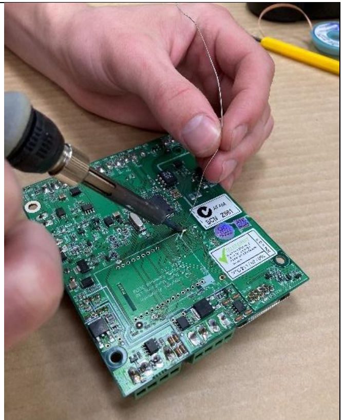
Solder both modem pins to the CTU Board
